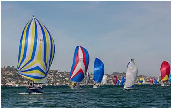
Spinnakers fall into three broad categories; Racing Asymmetric, Racing Symmetric, and Cruising. In each of those there are different options depending on the intended conditions, both wind speed and wind angle, which you want to use the sail in.
